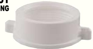
• The E-Z Nut is designed for hand tightening without tools. This is a distinct advantage particularly in confined spaces. The E-Z Nut's extra depth provides additional thread contact to prevent skipping.
